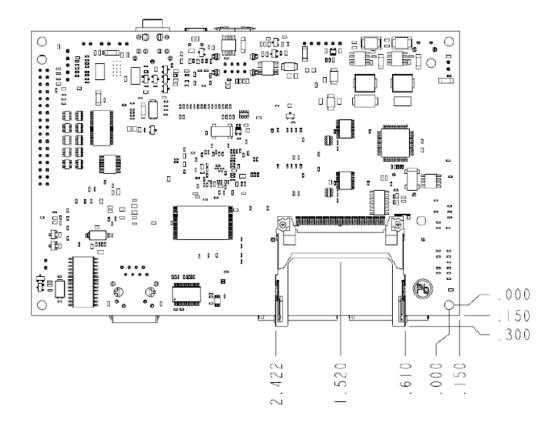
The final view illustrates the underside. Notice socket J2 is located on the underside.
