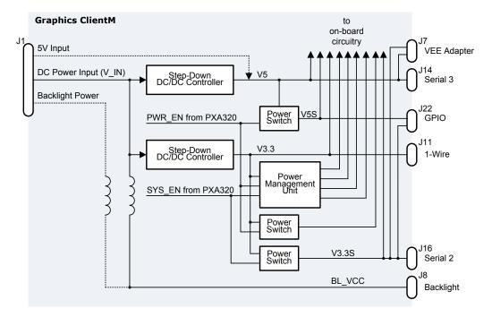
The GCM power supply is designed for high efficiency and low noise. It utilizes two highefficiency step-down DC/DC controllers to regulate the incoming DC power from J1, page 30 generating 3.3 V and 5 V. A multi-function, programmable power management unit provides additional power regulation generating all other voltages required by the onboard circuitry. For electrical specifications, see Power Supply Specification, page 46.
