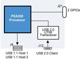
The second option provides a USB 1.1 host port on socket J4, a USB 1.1 client port on socket J12, and a CSI on socket J21. The CSI uses ten of the twelve GPIOs. In this option, only two GPIOs are available for application use on socket J21.
