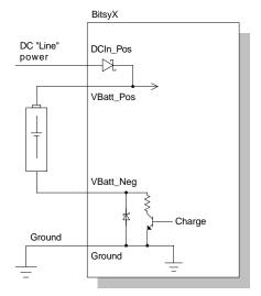
The Charge signal comes from the ADSmartIO controller (port PB0) and is also available on J3 pin 22 for external use. Writing a logic "1" to PB0 turns on the trickle charging. It is up to the application to manage battery charging.
