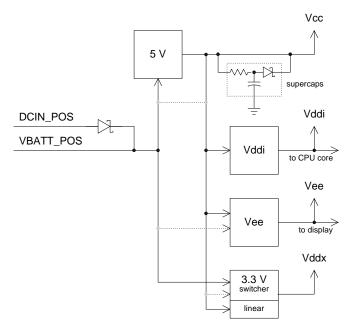
DC\_IN and VBATT voltages are mixed using a diode with a low forward voltage. This allows a battery and DC power supply to be connected at the same time. If only one power supply is used for your system, use the VBATT\_POS input. See sections 5.3.7 and 5.5.3 for examples.
