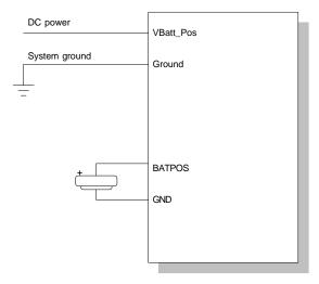
This diagram also illustrates how to connect a coin cell to the RTC circuit for systems that require the RTC to be maintained under all power conditions.
