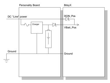
In this example, DC "Line" power may come from a DC power supply, battery or other DC power source.
