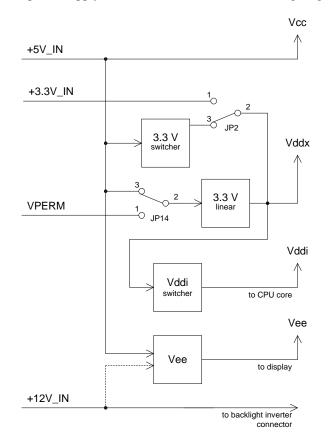
Vddi is a variable-voltage power supply controlled by the XScale  $I^2C$  bus (4.5.5, 6.2.2). This voltage scaling feature allows the operating system to manage power consumption over the full range of CPU clock rates.
