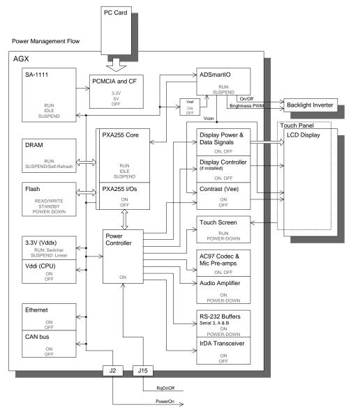
In the diagram, the power management modes of each subsystem are indicated in gray. Arrows indicate the direction of both signal flow and of power management.
