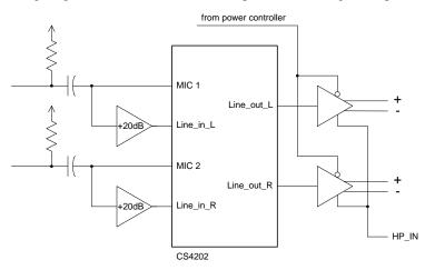
The AGX microphone circuitry can be factory configured to support "line in" inputs (1 Vrms with no electret pull-ups) and different input gain and filtering. If a special configuration needed for your project, consult ADS Sales with information about your requirements.
