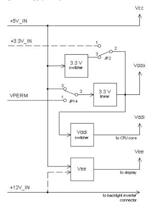
Vddi is a variable-voltage power supply controlled by the XScale I<sup>2</sup>C bus (4.5.6, 6.2.2). This voltage scaling feature allows the operating system to manage power consumption over the full range of CPU clock rates.
