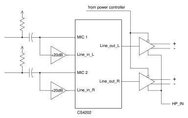
The VGX microphone circuitry can be factory configured to support "line in" inputs (1 Vrms with no electret pull-ups) and different input gain and filtering. If a special configuration needed for your project, consult ADS Sales with information about your requirements.
