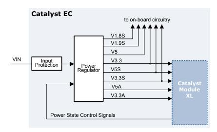
The architecture of the power supply partitions power distribution across the Catalyst Module XL and the Catalyst EC carrier board. The Catalyst EC requires a main power input VIN on header J5, page 32. The maximum main input voltage is limited by input protection. Configurations for higher voltage inputs are available as volume production options. For further details, see Power Supply, page 48.
