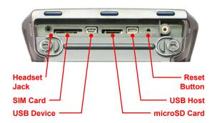
To access the I/O panel, remove the protective cover located on the bottom side of your Zypad WL15xx.
