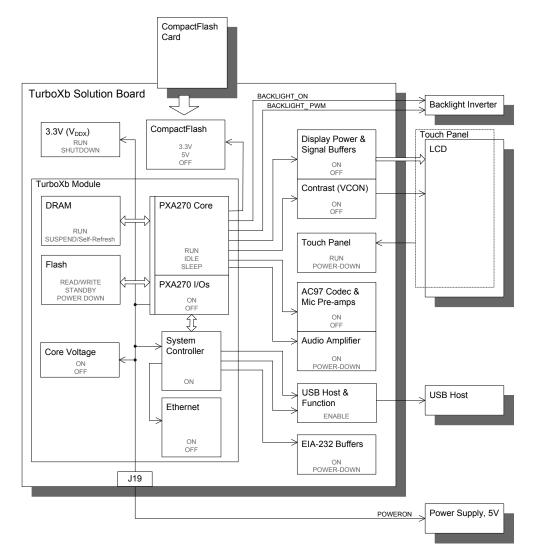
In addition to disabling select subsystems, the TurboXb development system supports sleep operation through control of its on-board peripherals and power supplies. The signal POWERON can control an external power supply. See <u>J19</u>: <u>Input Power</u>, page <u>37</u>. The system negates this signal when entering Sleep mode. See <u>Power Specification</u>, page <u>39</u> for electrical specifications.
