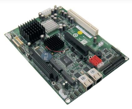
The ALUDRA processor board provides all the benefits of Intel's new Atom LPIA architecture in a EBX form factor.
