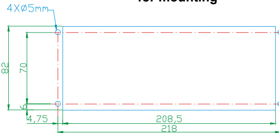
Required cut-out dimensions for mounting
