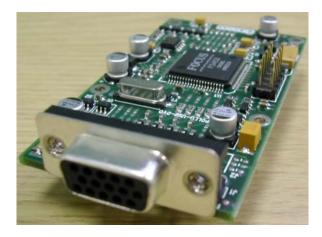
The VGA Card converts APOLLO high-resolution DVO (digital video output) to analog CRT outputs, from VGA to SXGA resolutions. The following image shows the VGA card in position:
