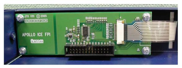
The Front Panel Interface is 'stacked' on the back of the LCD and has the tail from the front membrane plugged into a ZIF socket.
