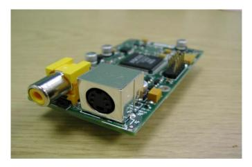
The TV Card converts APOLLO high-resolution DVO (Digital Video Output) from VGA to SXGA resolutions, and produces standard analog television (SDTV) output to S-Video and composite video connector outputs. The following image shows the TV card in position:
