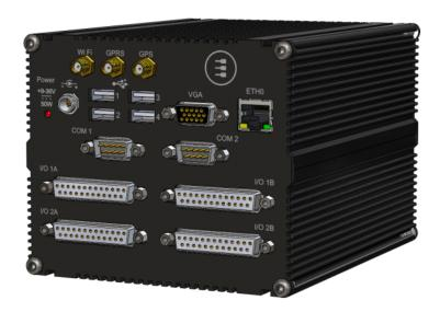
The ISIS Industrial Compact Enclosure (ICE) encloses a special build version of the ISIS Single Board Computer (SBC). The ISIS has been modified so that it can plug directly into the ISIS ICE interface PCB thereby transferring essential interconnection signals such as USB, Ethernet, RS232 and power to the front panel connectors. The ISIS ICE also protects the ISIS, and provides a CE-compliant product for use straight out of the box.
