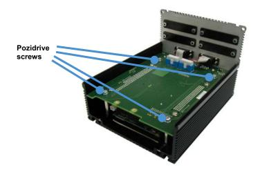
5. Place a medium sized flat bladed screwdriver into the space between the ISIS heatsink and the top extrusion and twist to free the heat pad from the extrusion:
