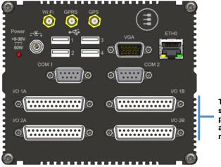
The I/O connectors shown here are optional positions, available in addition to those on the rear panel.
