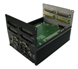
3. Remove the four remaining M4 fixing screws on the front and rear plate.
