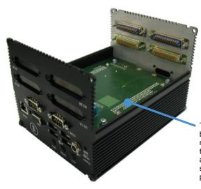
The version of the ISIS baseboard shown here does not have the PC104 stack through connectors fitted for additional PC104 cards. The stack through version of this part will be supplied.
