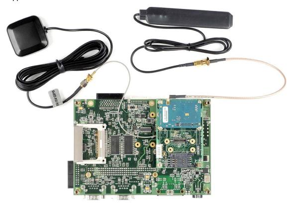
The modem interfaces connect to the PXA270 serial ports and can be accessed and configured in Linux as standard serial ports. In addition to this, there are also a number of control/status GPIO signals connected to the module interface, J23. These can be accessed through a GPIO Expander, MAX7313, which is connected to the I<sup>2</sup>C interface.
